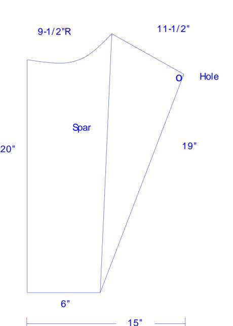
Lay a plastic trash bag flat out on a table Make a cardboard template or measure and cut. The 20" line goes along the folded edge of the trash bag.
