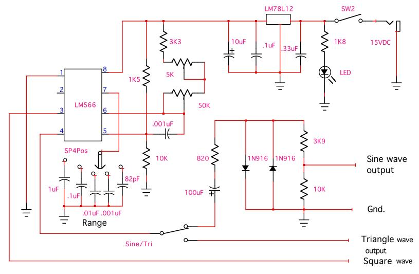
The LM566 is a voltage controlled oscillator. It will produce a square wave at pin 3 and a triangle wave at pin 4. Additional components convert the triangle wave to a sine wave. the 50K pot is frequency adjust and the 5K pot is fine adjust.
