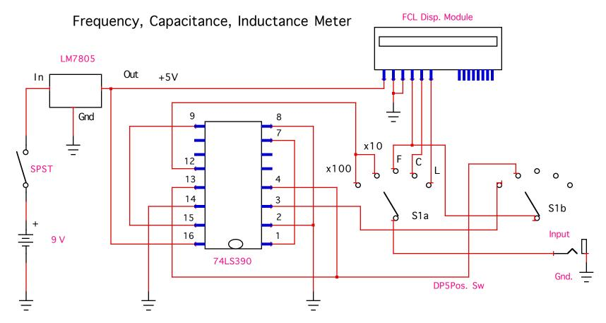
The FLC display module is a stand alone unit which will measure frequency only up to 500kHz, due to a manufacturing defect. The 74SL390 decade counter is connected for frequency division of 10 and 100, providing a theoretical reading of up to 5mHz or 50mHz. S1a and S1b are connected to provide for C and L readings as well as the three readings for frequency.
