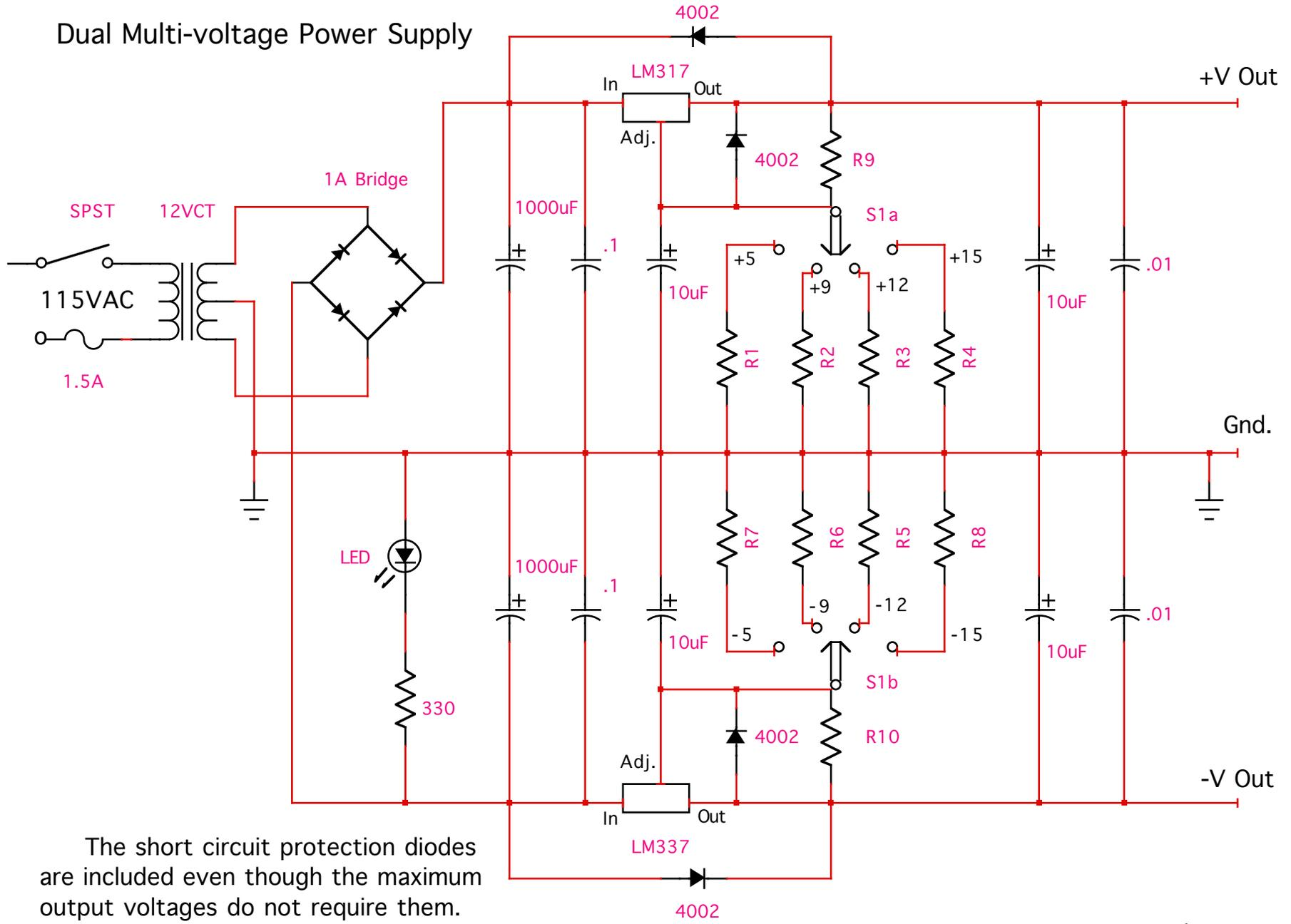
The short circuit protection diodes are included even though the maximum output voltages do not require them.
